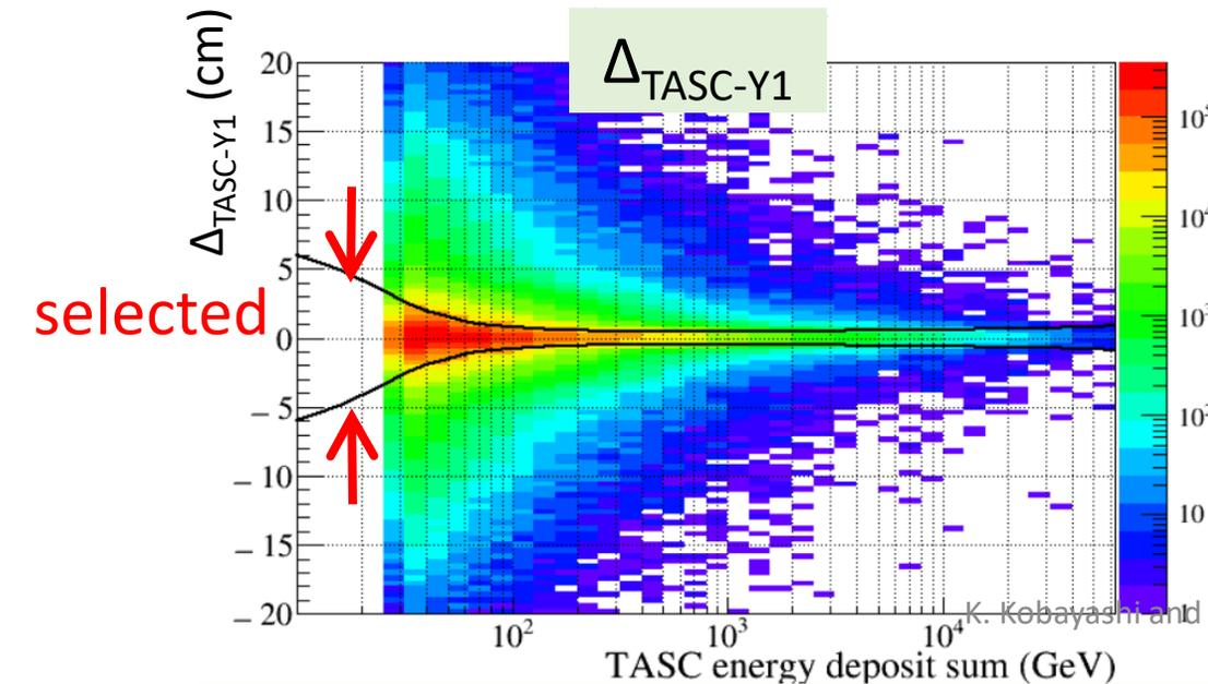
In order to remove residual mis-reconstructed events, track reconstructed in IMC is checked using TASC energy deposit.
