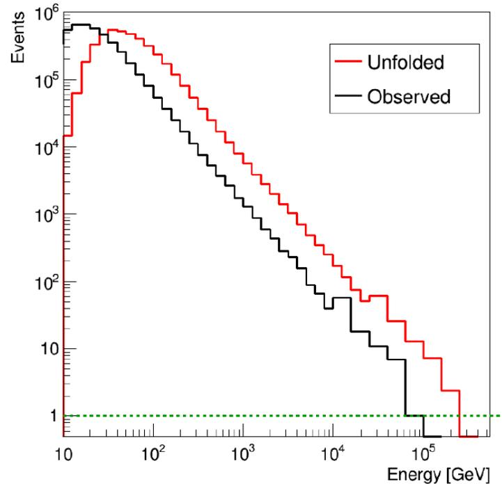
The energy resolution of proton is 30-40%. Therefore, we apply Bayes unfolding to reconstruct energy.
