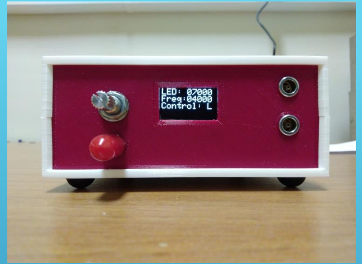
Stand-alone desktop module of fast light pulses source
