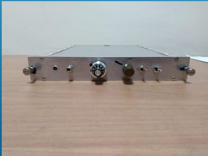
NIM module of fast light pulses source
