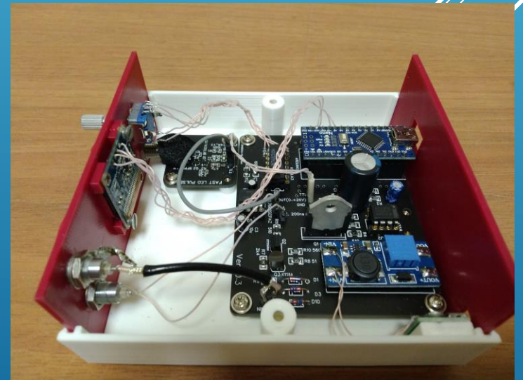
Stand-alone desktop module of fast light pulses source
