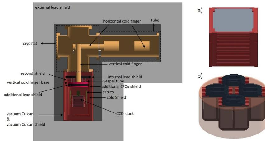
Left: latest simulated detector design. The thickness of the external lead shield is 20 cm. The electro-formed copper components are shown in red, while the OFHC copper ones in yellow. Right: zoom on different CCD stacks. a) Horizontal CCD stack. b) Vertical CCD stack. The gray parts are the CCDs, the red parts the copper holders
