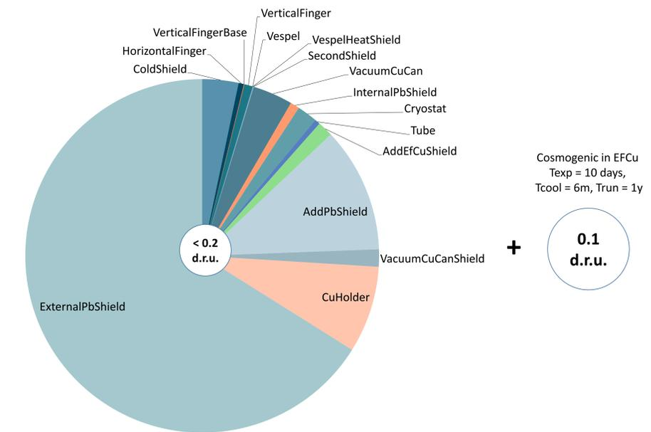
Contribution to the background rate of each detector component. The horizontal CCD stack design was used. The total background rate is less than 0.3 decays/kg/keV/day [d.r.u.]. Texp: exposure time to cosmic rays, Tcool: time spent underground before data taking, Trun: experiment running time. For the OFHC Cu components: Texp = 3 m, Tcool = 6 m, Trun = 1 y.
