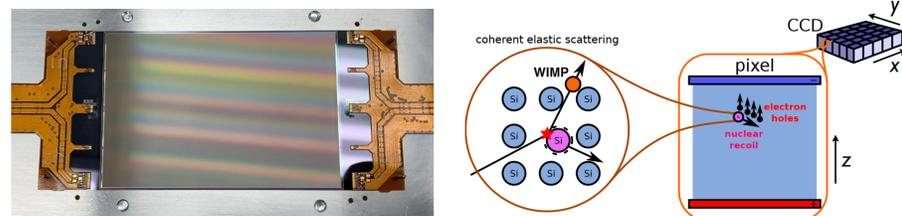
Left: tested 6k x 4k pixels CCD wire bounded to a kapton cable. Right: Principle of a dark matter detection in a CCD. A WIMP scatters with a silicon nucleus or electron producing ionization in the CCD bulk. The charge carriers are then drifted along the z-direction and collected at the CCD pixel gates [1].
