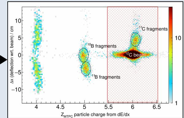
Resultant fragments separated by  $dE/dx$  in the main detector
