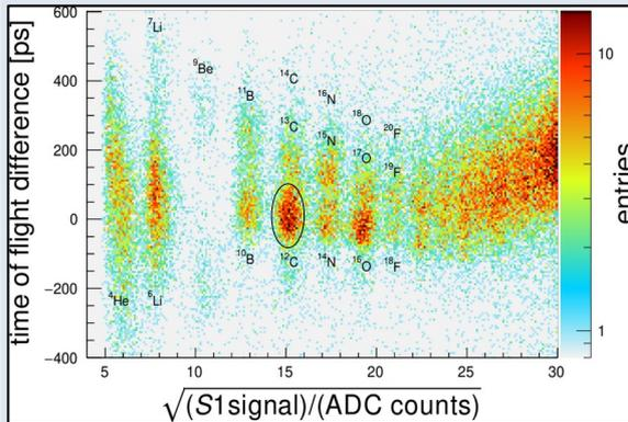
Secondary ion beam composition at NA61/SHINE emerging from H2 beam line
