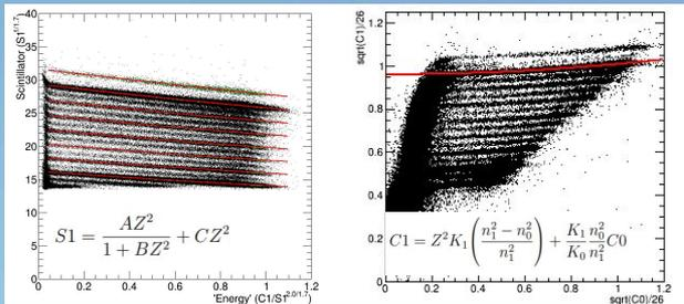
→ A low-energy (left) and a high-energy (right) charge assignment method is used to extrapolate the Z dependence of detector signals to higher signal space, where high-Z events appear but charge bands are not visible.
