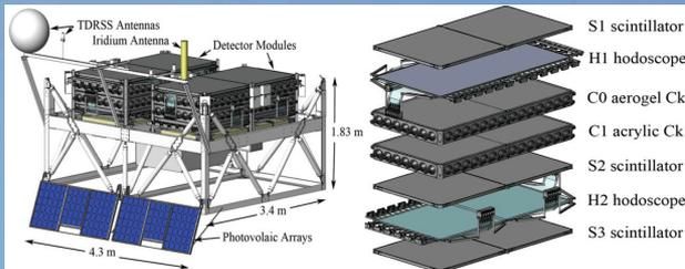
→ SuperTIGER (Super Trans-Iron Galactic Element Recorder) is designed to measure ultra-heavy galactic cosmic rays (GCR) and probe their source and acceleration mechanism.
