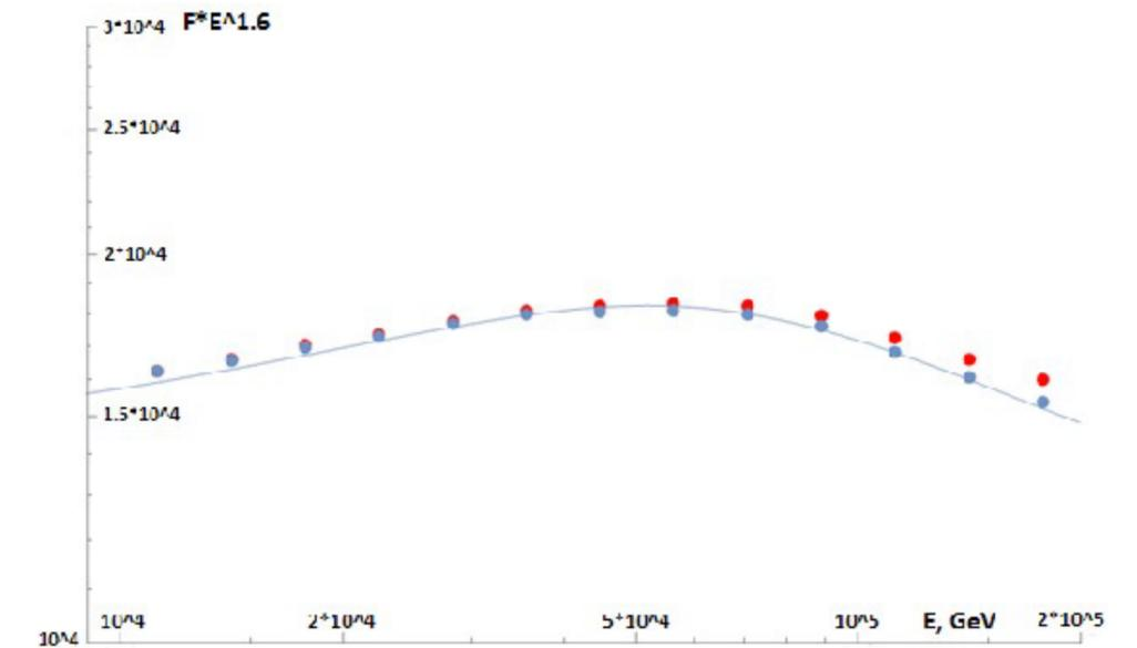
Predictive model of all particle spectra for a source with minimum  $\chi^2 \sim 3$  at a distance of 170 parsecs and an age of 4000 years and experimental data. Red point -HAWC data Blue point- HAWC data multiplied by the correlation function
