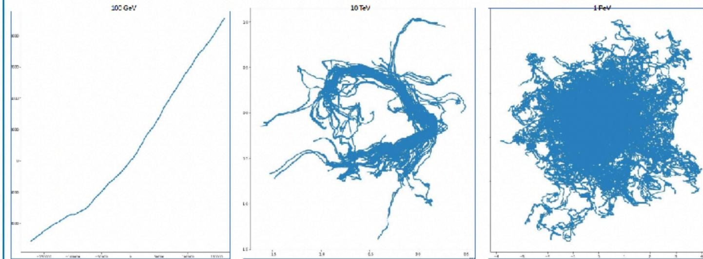
Trajectories of particles with energies of 100 GeV (not to scale), 10 TeV and 1 PeV in turbulent magnetic field  $B_{\text{random}} = 6 \mu\text{G}$  and  $B_{\text{mean}} = 6 \mu\text{G}$  (directed along the Z axis). From these trajectories it can be seen that for energies below 10 TeV the anisotropy is determined by the local field
