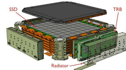
*Silicon strips (precise tracking) + tungsten converter (pair production)*
