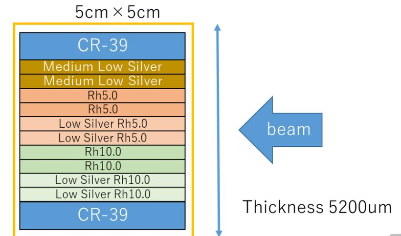
Fig.3 Detector consists of emulsion and CR-39.
