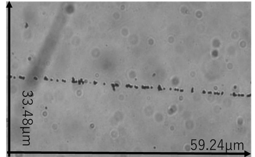
Fig2. Tracks generated by irradiating a low-sensitivity nuclear emulsion with a carbon beam
